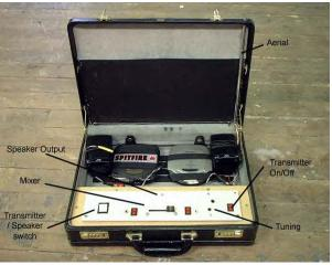
We are admittedly dunces when it comes down to ther ins and outs of electronic know how, however using the circuit below and following our list of which components are placed where, you should be able to produce your very own transmitter.
